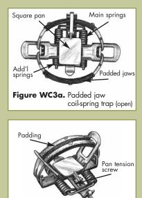
Figure WC3b. Padded jaw coil-spring trap (closed)
